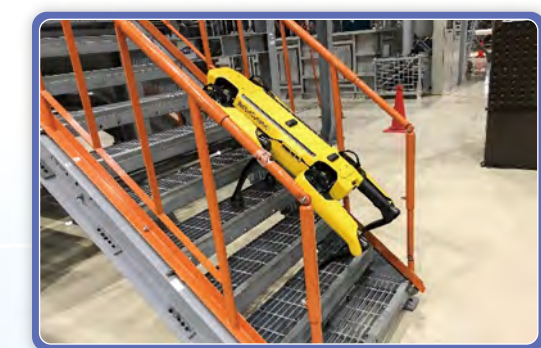
Travelling performance test for a quadruped walking robot Ascending/descending performance test using Mock-up Stairs whose tilt angle, handrail width and board material can be changed
