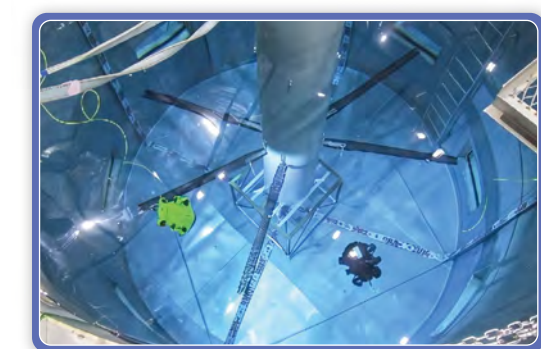
VT inspection using an underwater drone Simulation test in which a 30-ton overhead traveling crane collaborates with a water tank with an underwater drone submerged in the tank
